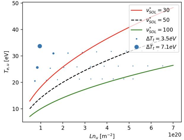
Figure 1: *Difference in target temperature for SOL simulations with kinetic vs. fluid electrons.*
