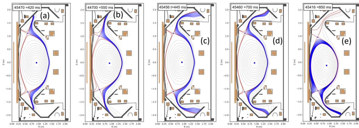
Figure 3 – A selection of some of the magnetic topologies obtained during the first MAST-U campaign. (a) Double null conventional divertor (b) Double null X-divertor (c) Double null Super-X divertor (d) Double null extended leg divertor (e) Disconnected double null extended leg divertor
