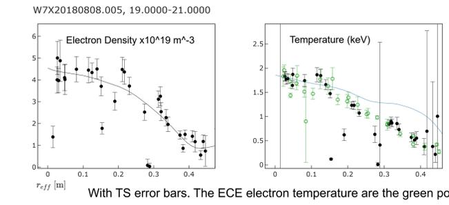
With TS error bars. The ECE electron temperature are the green points
