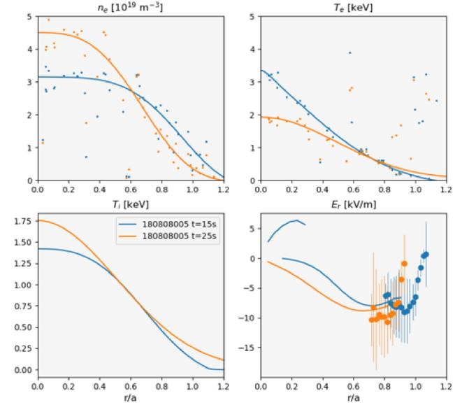
Thomson, X-ray crystal spectrometer, and PCR ( $E_r$ ) profiles
