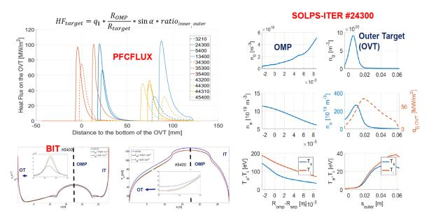
The heat flux footprint predicted by the geometric model from PFCFLUX [12] differs significantly from the one calculated by the SOLPS-ITER (represented in the right figure for scenario #24300) fluid model or the BIT [17] PIC code indicating the likelihood of a large radiated fraction (46% for #5400 in BIT simulation) or quasi-detached plasma (SOLPS).
