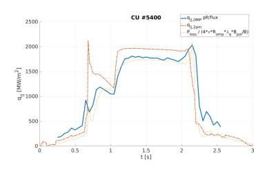
SOL conditions influence the separatrix conditions. In particular, the sheath-limited 2-point model [11] can be simplified to yield:
