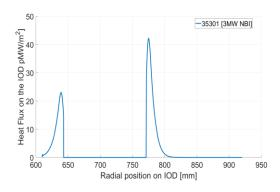
Fast ions and fast neutrals losses for two possible I-mode configurations. The deposition and additional losses due to the Toroidal Field Ripple (TFR) and the Charge-Exchange (CX) with edge neutrals are given by the EBdyna code [15]. The heat flux on the Open Divertor in the USN configuration is large, making only a brief full-power I-mode possible in the clockwise field and current configuration (#35301): this could however be used as a way to enter Super H-mode [16].
